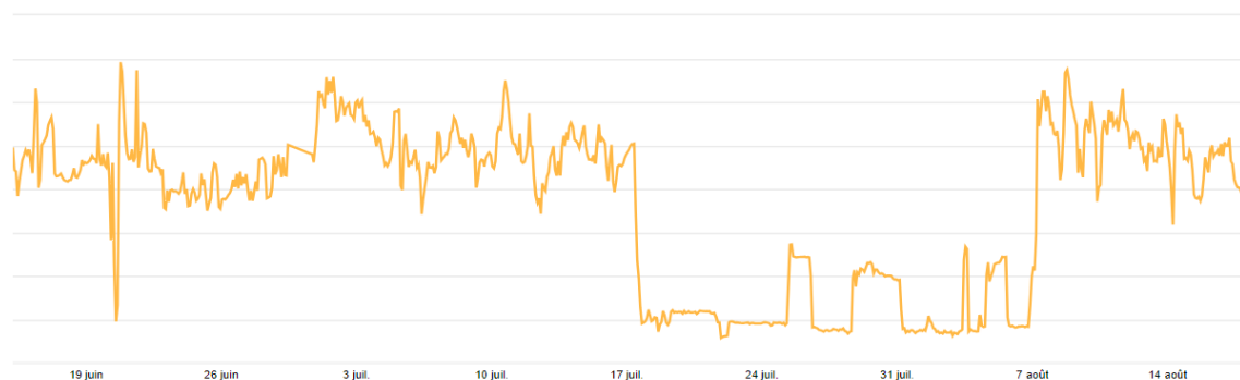
Figure 13. Steam consumption before, during and after the first shutdown.
