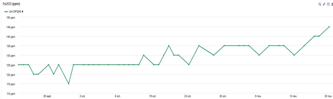
Figure 17. Second shutdown results: iron in hydrate (scale of Y-axis [110-150 ppm]).
