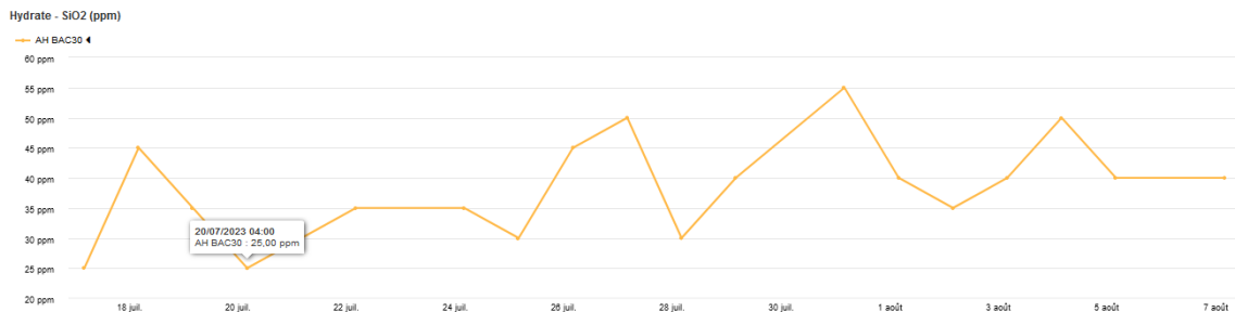
Figure 12. First shutdown results: silica in hydrate (scale of Y-axis [20–60 ppm]).
